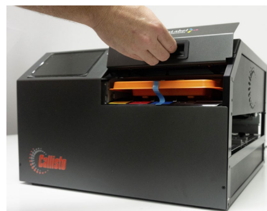
Pull out orange ink cap and blue tape.
