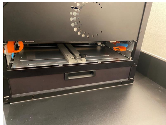
Pull out left/right orange sled caps and blue tape.
