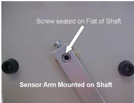
Place the Sensor Arm over the Sensor Arm Shaft End so that the Flat on the Shaft is positioned under the Screw. Using a small screwdriver tighten the Sensor Arm Screw snugly onto the Flat on the Sensor Arm Shaft.
